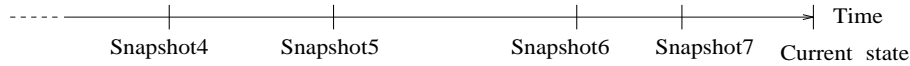
Figure 11.1: Snapshots represent consistent database states as of some time in the past.
