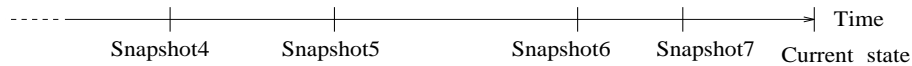
Figure 2: Snapshots represent consistent database states as of some time in the past.
